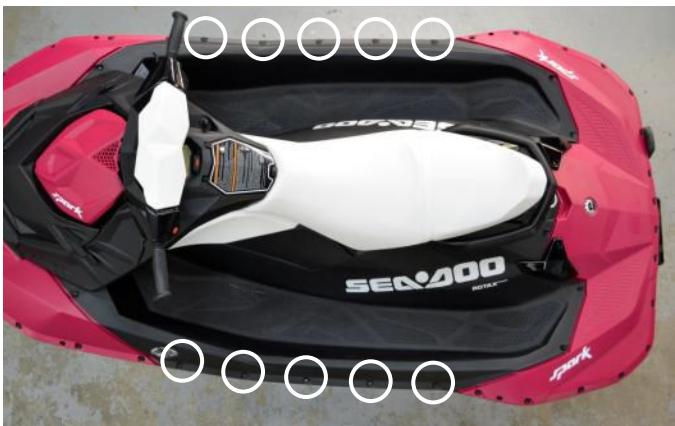
Discard plastic washers. Reinstall Torx bolts, upgraded washers in place of plastic washers, and nuts. **NOTE: Torque bolts to 31 in•lb (3.5 N•m).**
