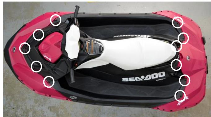
Discard plastic washers. Reinstall Torx screws with upgraded washers in place of plastic washers. **NOTE: Torque screws to 49 in•lb (5.5 N•m). DO NOT apply thread locking agent.**
